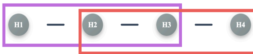
Figure 9: Linear H_4 chain with 2 fragment approach. Algorithm includes overlapping 3 atom fragments. ( H_1, H_3 centered on H_2 and H_2, H_4 centered on H_3 )
